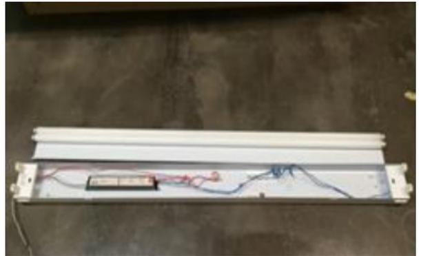
4. Break the mate on the yellow disconnect to cutoff the ballast from the line wires.
